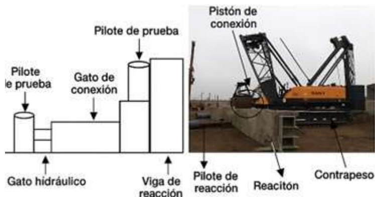
Figure 3: Diagram of the lateral load test and reaction mechanism.
